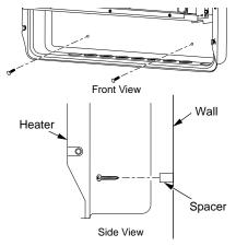
Figure 12 - Installing Bottom Mounting Screws
